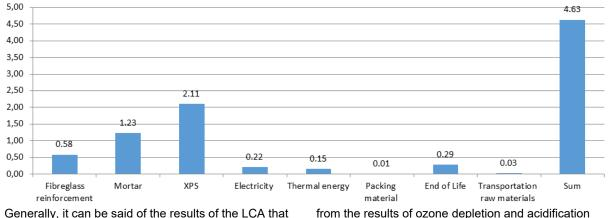
Generally, it can be said of the results of the LCA that the provision of the pre-products (Module A1) makes the greatest contribution to environmental effects. Above all the XPS has the greatest influence on a large part of the impact categories examined, especially on the global warming and ozone formation potential.
