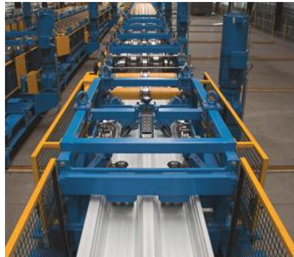
Pic. 1: Rollforming of a trapezoidal sheet
