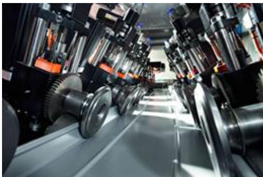
Pic. 1: Rollforming of a trapezoidal sheet
